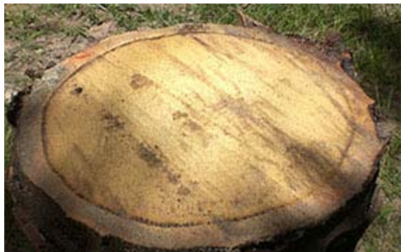
Figure 6. Oil palm trunk at transverse section consists of the main part of the trunk, cortex and bark.
