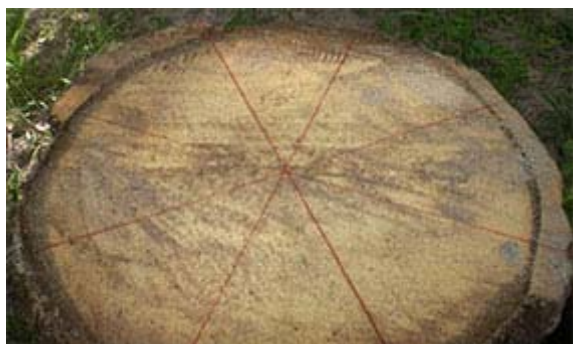
Figure 7. Sawing patterns were called cobweb sawing.
